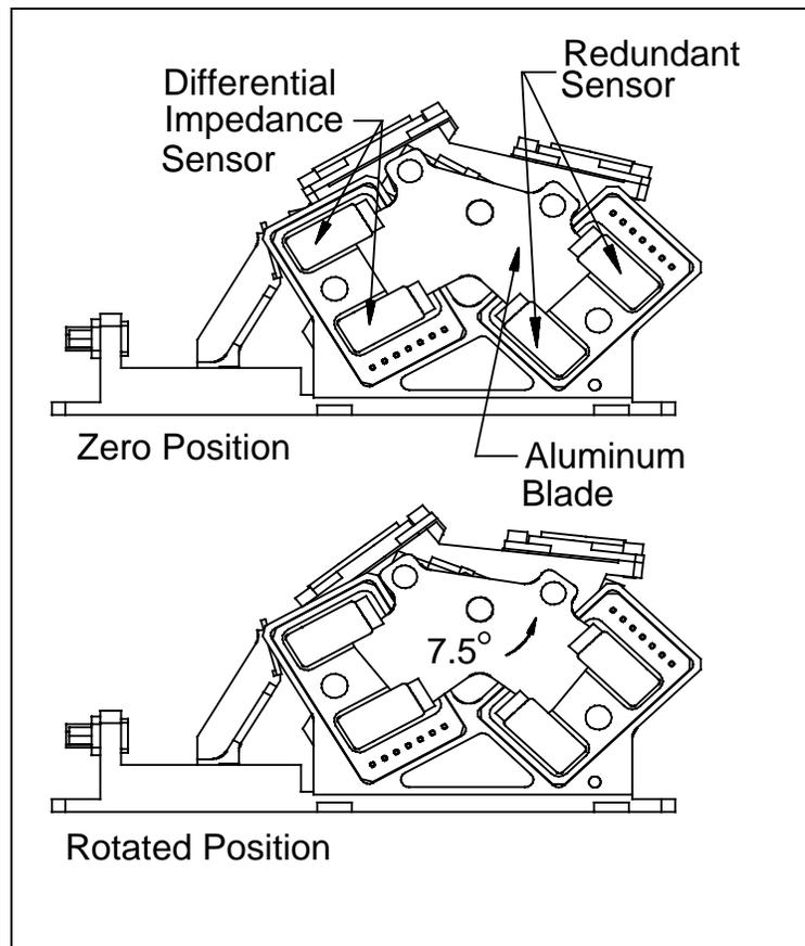
**Figure 4. CSMM Position Sensor**
